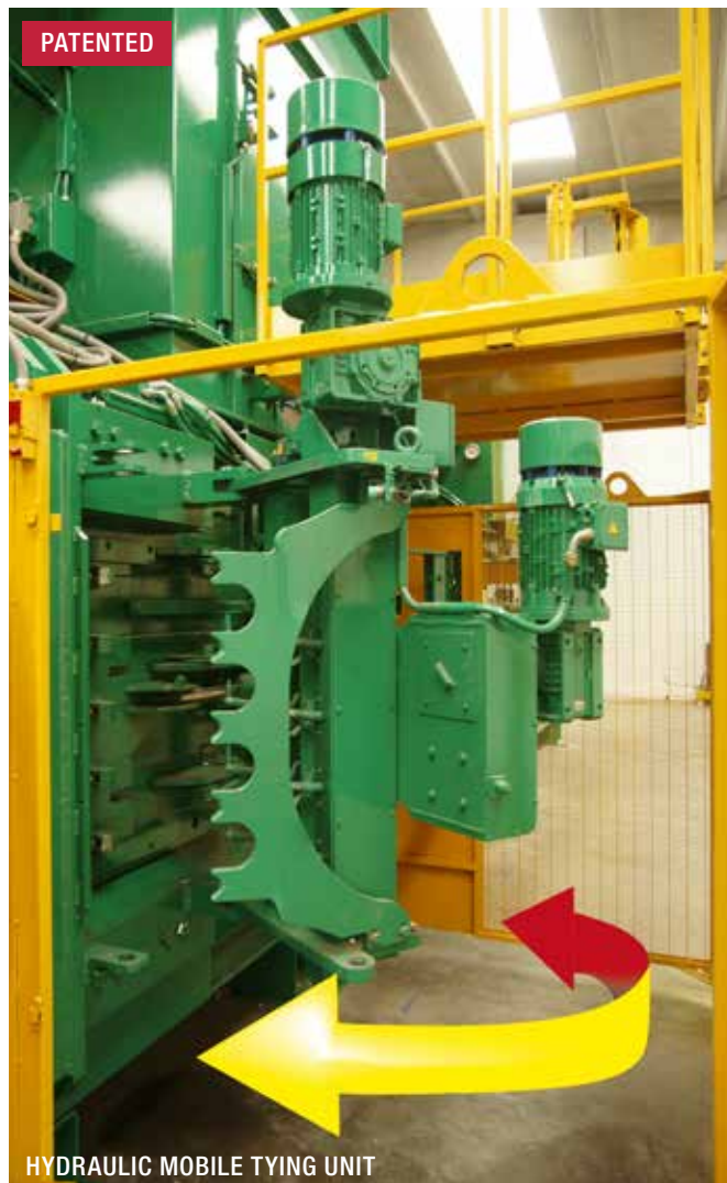
HYDRAULIC SIDE DOORS FOR WIRE TYING UNIT PROTECTION
