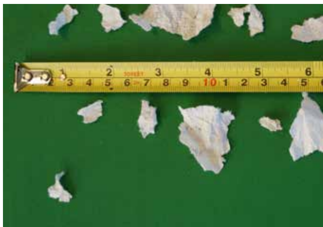
SHREDDER MAC 1500 D GRIDS 38 MM
