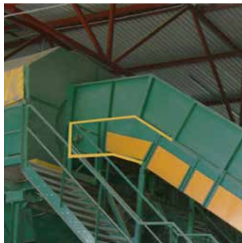
MOTORIZED HEAD PULLEY SECTION WITH 30° INCLINATION
