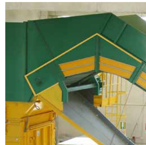
MOTORIZED HEAD PULLEY SECTION WITH 60° INCLINATION
