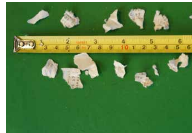
SHREDDER MAC 1500 D GRIDS 28MM
