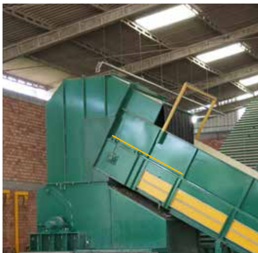
MOTORIZED HEAD PULLEY SECTION WITH 0° INCLINATION
