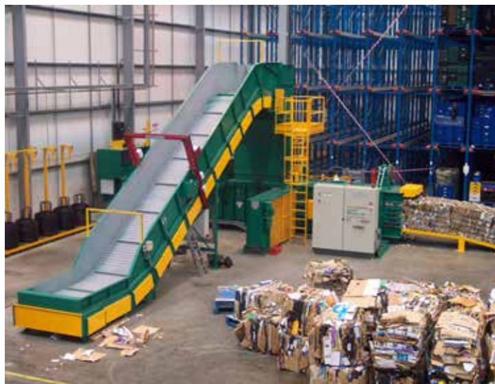
LOADING SECTION OUT OF PIT
